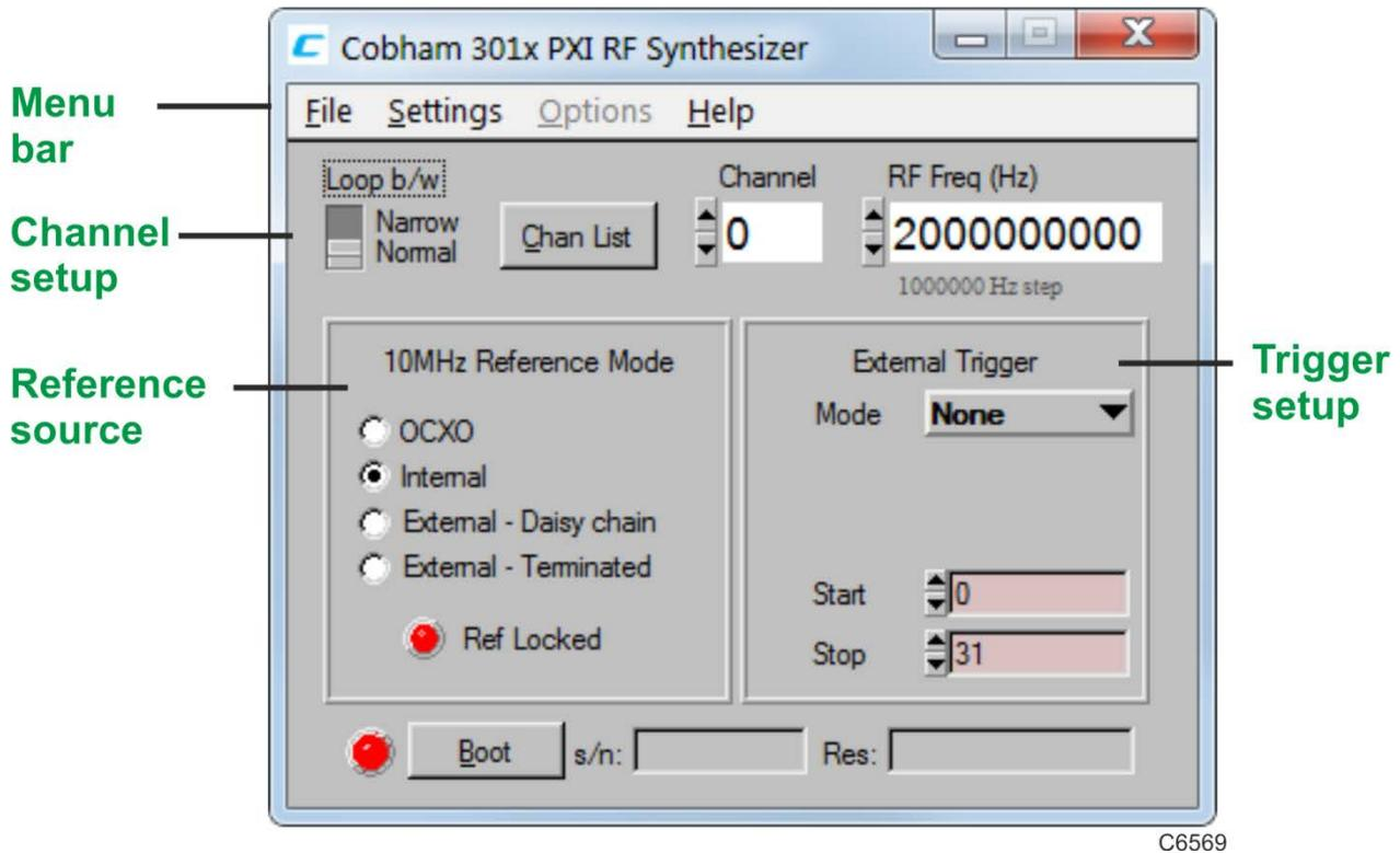
Fig. 3 Synthesizer soft front panel (3010 is similar)
