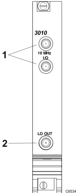
1 10 MHz I/O Two SMA I/O sockets in parallel.
