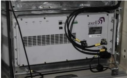
A D-OBR onboard the train
